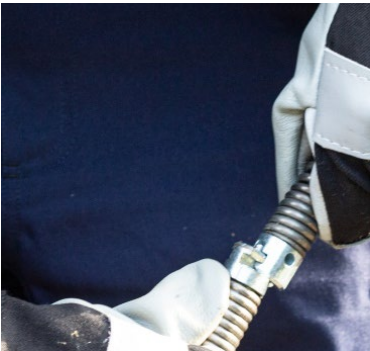
Fig. 4: Fixing the drill head with the snap-lock
