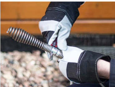
Fig. 5: Releasing the snap-lock to separate the drill head from the cable.
