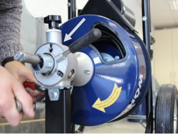
Fig. 10: Automatic feed unit marked by grey arrow
